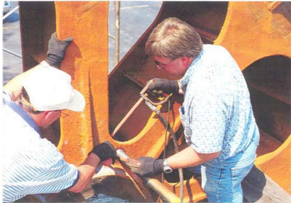
Fig. 3.1 – Magnetic particle testing of sheave spokes using prods
