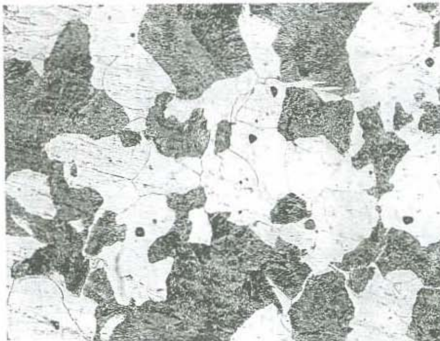
Figure 26 - Microstructure of the Sheave. [Mag. 200X] Top) Sample #3 Bottom) Sample #4
