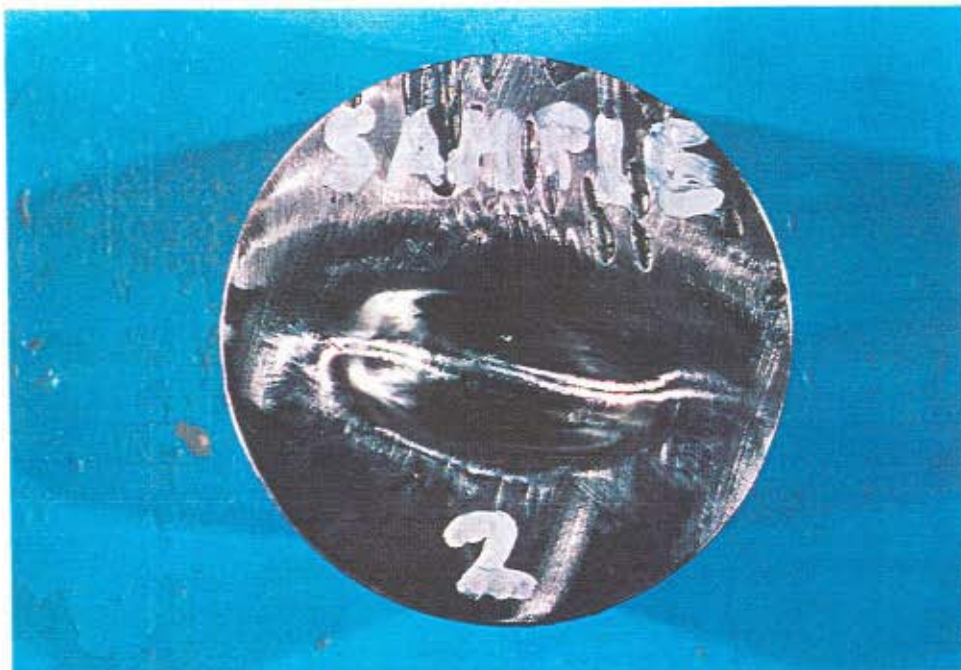
Figure 7 - Sheave Wheel Core Sample #2. The Surface Crack Detected Was Ground to Gauge Crack Depth Prior to Coring. (4/99/14-8)
