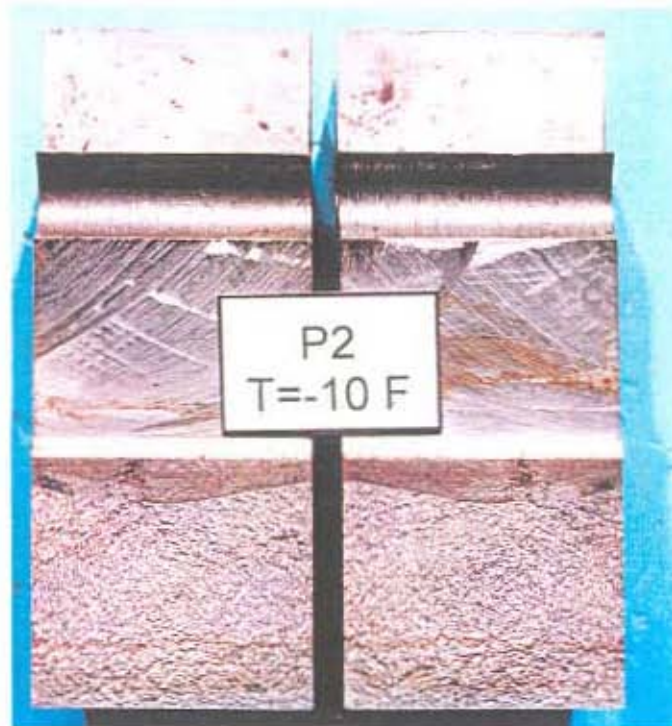
Figure 32 - Fracture Surfaces of Test Specimen P2. (6/00/3-5)
