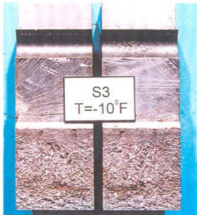
Figure 42 - Fracture Surfaces of Test Specimen S3. (6/00/3-7)
