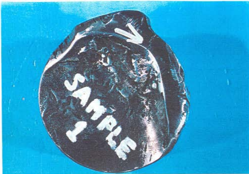
Figure 6 - Sheave Wheel Core Sample #1. Note Surface Crack Indicated by Arrow. (4/99/14-11)
