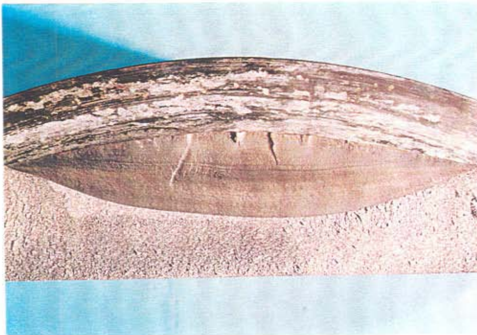
Figure 46 - Semi-elliptical fatigue crack extension from machined radius at trunnion shoulder (City of Duluth, MN Lift Bridge) (5/97/15-7)
