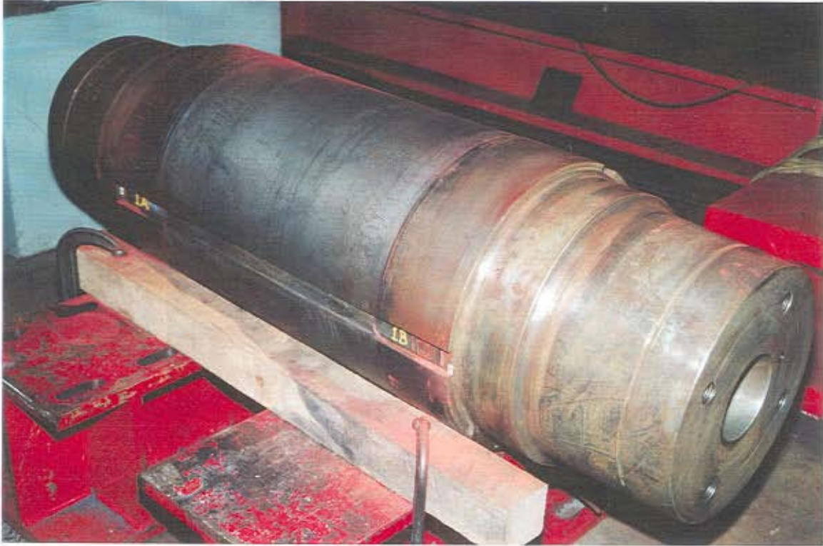
Fig. 3.4 – Trunnion after removal from sheave and prepared for NDE
