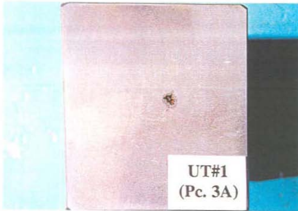
Figure 21 - Internal Trunnion Defect Detected By Ultrasonic Inspection (UT1). (12/99/7-4)
