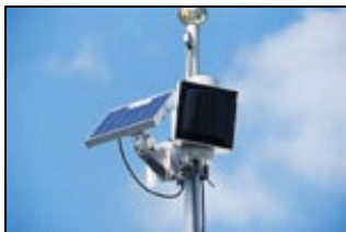
Solar powered transponder reader
