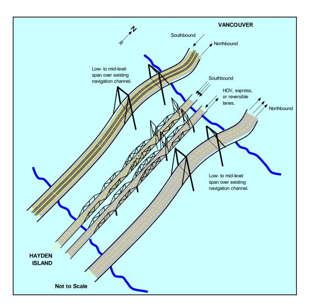
**Concept 7:** 8-lane freeway concept plus new LRT bridge with two-lane arterial
