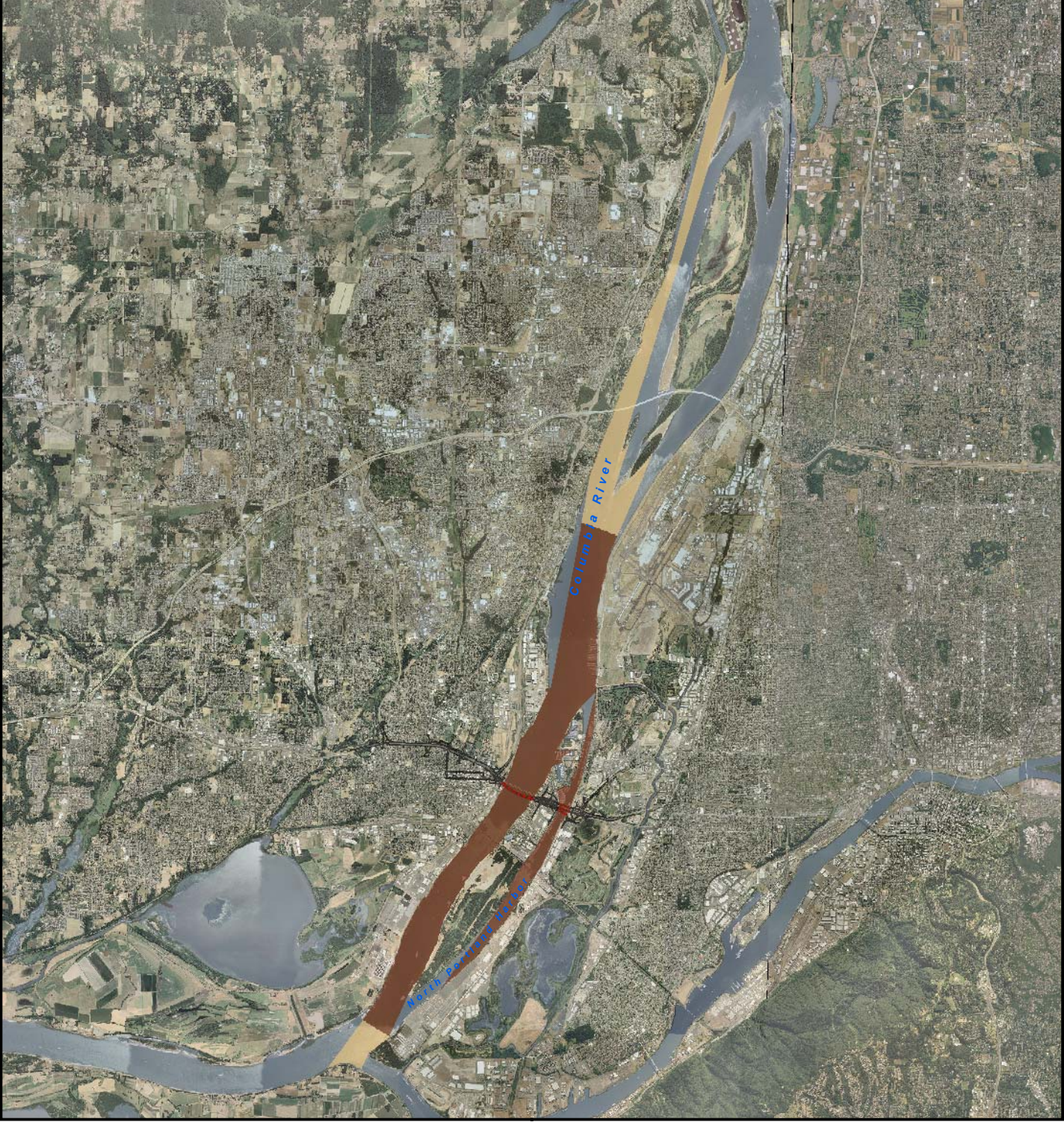
Figure 6-47. Extent of underwater vibratory pile-driving noise exceeding 120 dB RMS disturbance threshold for Steller sea lions
