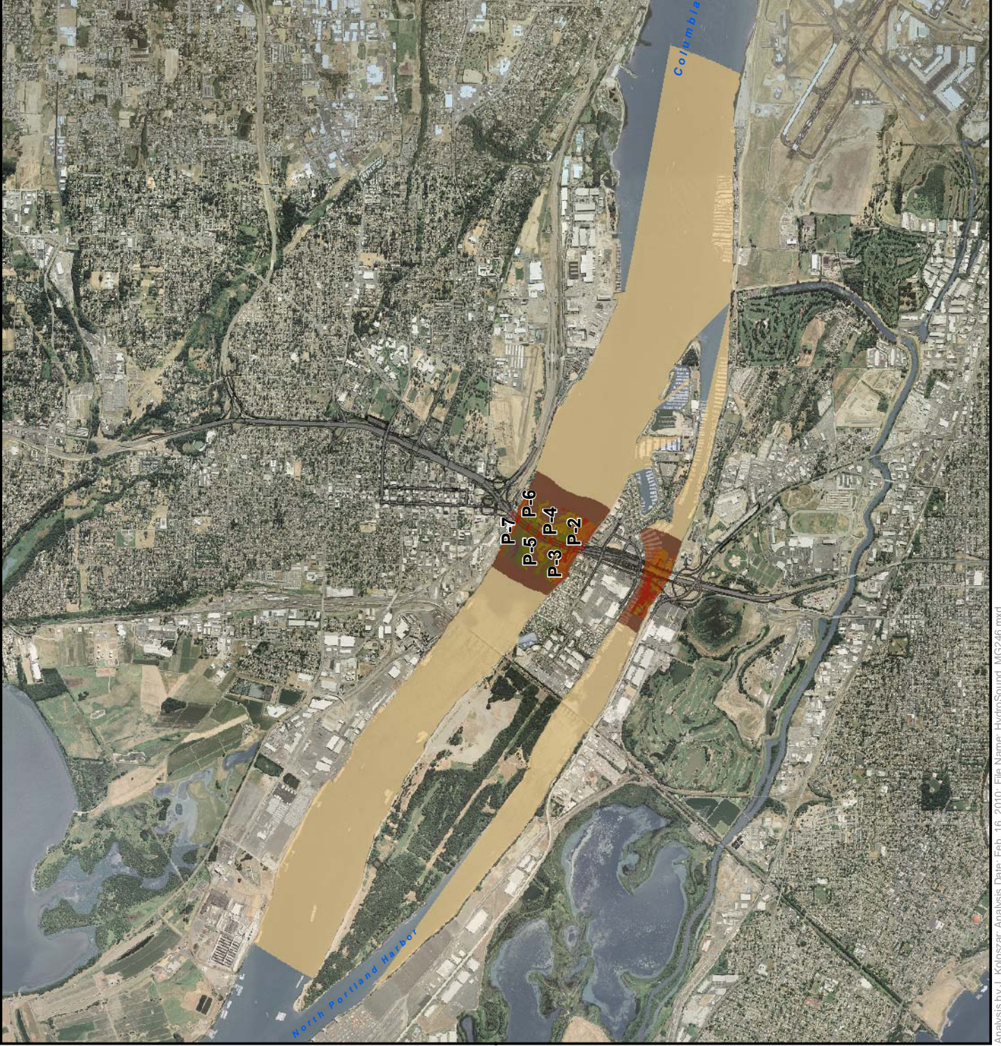
Figure 6-46. Extent of underwater impact pile-driving noise exceeding 160 dB RMS disturbance threshold for Steller sea lions, 36 to 48-inch pile
