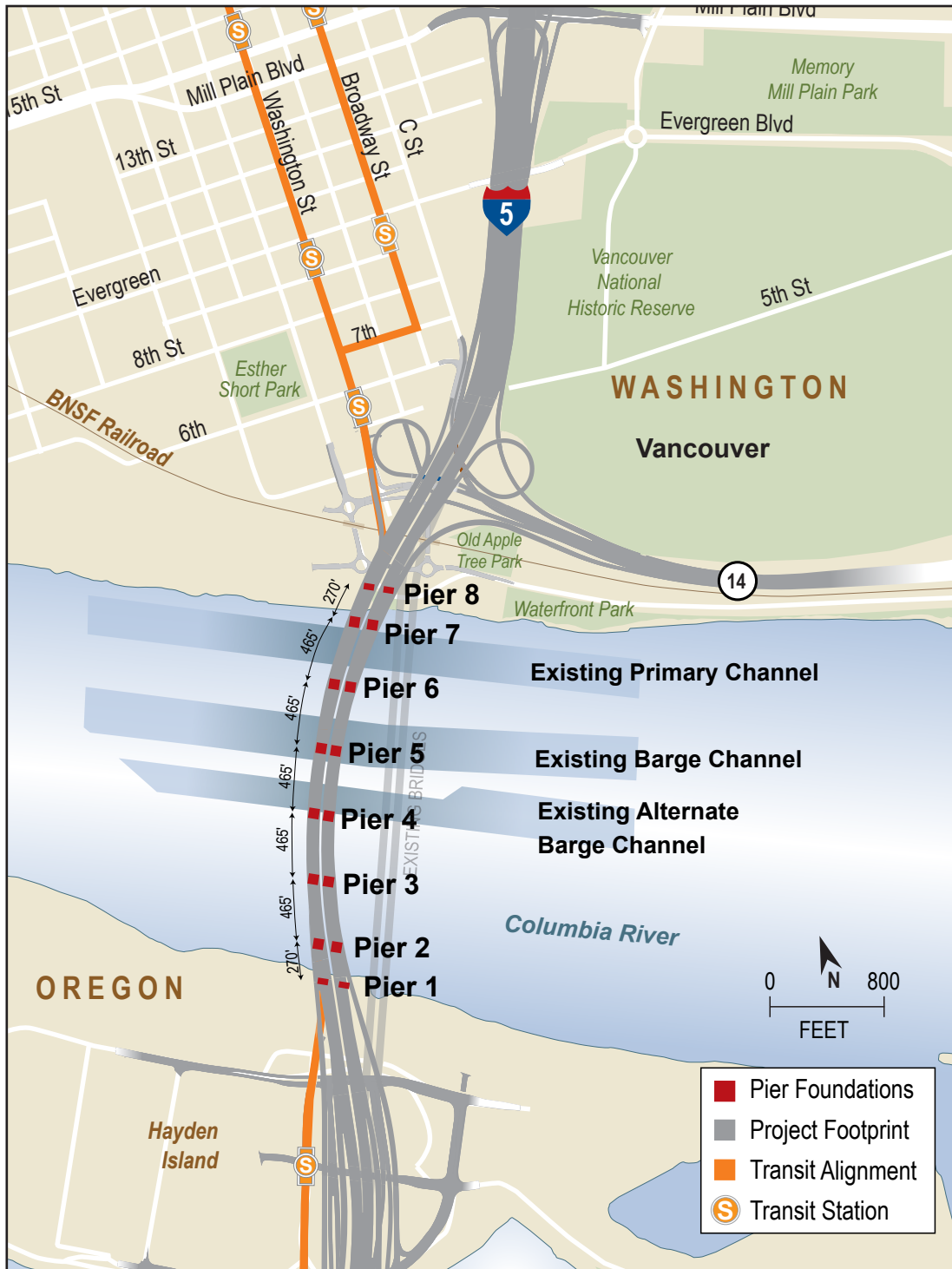
Figure 3-3. Proposed Layout of Columbia River Bridge Showing Piers and Existing Navigation Channels
