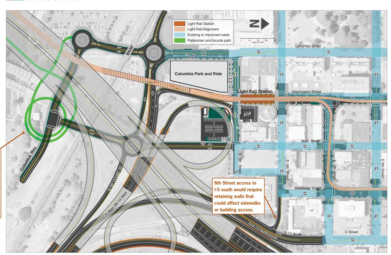
Pedestrian and bicycle path increases in length by 700 feet at a 115' bridge height. Average path grade is 3.5% at a 115' bridge height.
