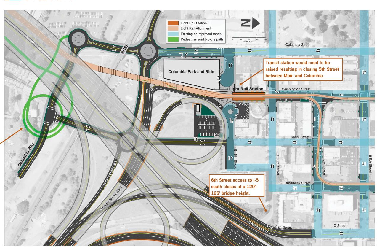
Pedestrian and bicycle path increases in length by 700 feet at a 120'-125' bridge height. Average path grade is 3.7% at a 120' and 4.0% at 125' bridge height.
