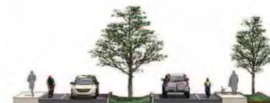
Street concepts showing planters for trees, parking for cars, bike lanes, and sidewalks for pedestrians.
