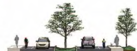
Street concepts showing planter for trees, parking for cars, bike lanes, and sidewalks for pedestrians.
