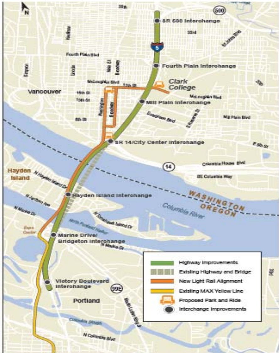
Figure 1. Alignments of the proposed Columbia River Crossing highway improvements, bridges, and light rail features.
