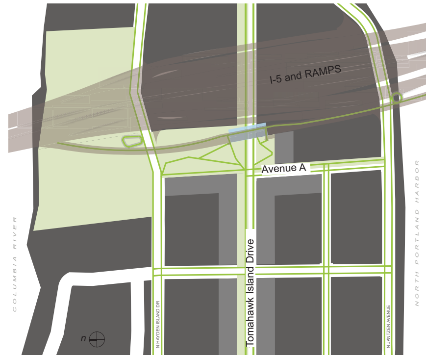
The Elevated Station Concept: Hayden Island Study Area. LPA freeway and LRT station are approximately 124 feet from Avenue A. (Source: ZGF)
