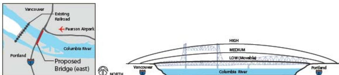
Figure 5-6. Supplemental Bridge Upstream/Low Level/Movable
