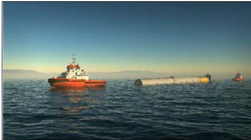
Figure 7. Tow of a spar platform for a floating wind turbine (Hywind)
