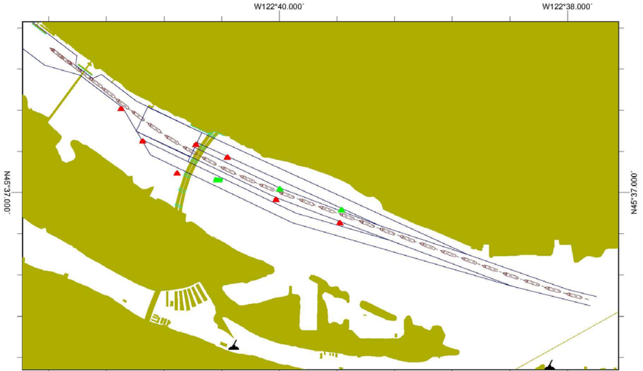
Figure A - 21: Run 21, 27-ft Channel, Sulphur Guardian Ballast (453ft x 75ft x 19ft) Upbound 2-yr River Flow, Wind S 15 Knots, Pilot A, Proposed CRC Primary Span
