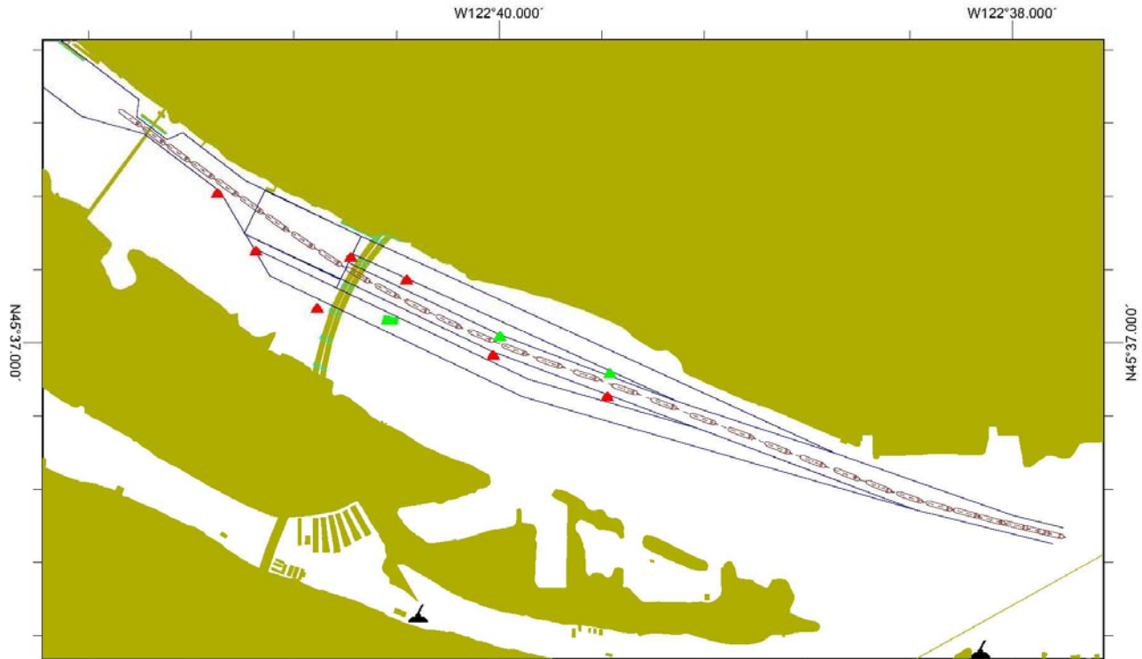
Figure A - 15: Run 15, 27-ft Channel, Sulphur Guardian Loaded (453ft x 75ft x 25ft) Downbound 2-yr River Flow, Wind S 15 Knots, Pilot A, Proposed CRC Primary Span
