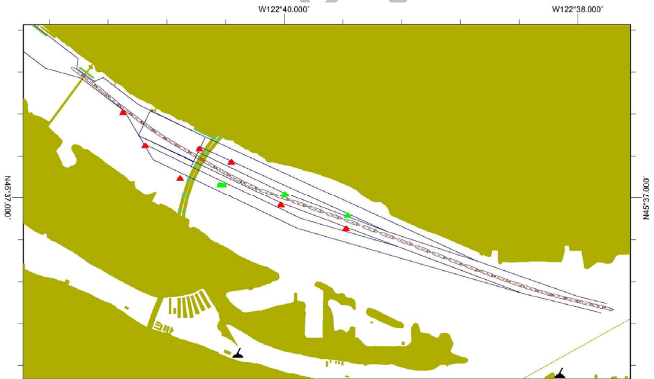
Figure A - 14: Run 14, 27-ft Channel, Sulphur Guardian Loaded (453ft x 75ft x 25ft) Downbound Normal River Flow, Wind S 15 Knots, Pilot B, Proposed CRC Primary Span
