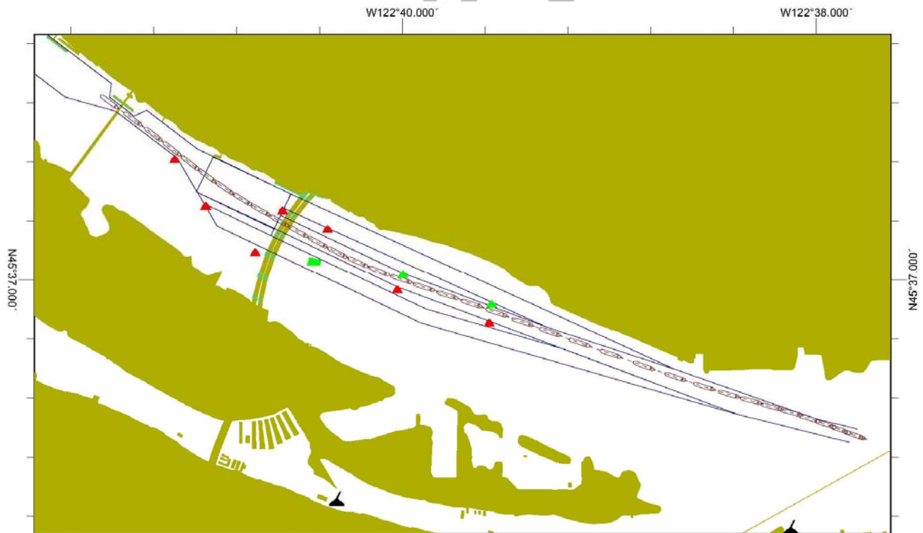
Figure A - 18: Run 18, 27-ft Channel, Sulphur Guardian Ballast (453ft x 75ft x 19ft) Downbound Normal River Flow, Wind S 15 Knots, Pilot B, Proposed CRC Primary Span
