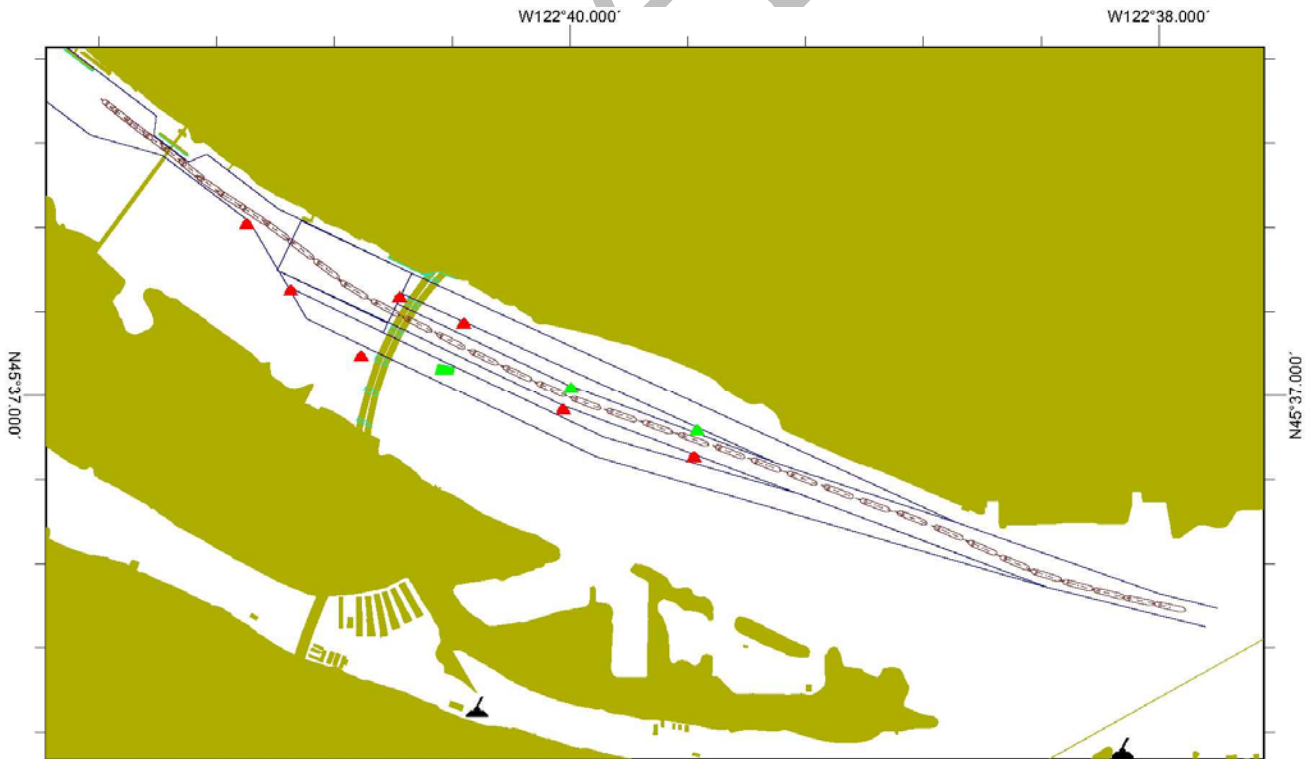
Figure A - 12: Run 12, 27-ft Channel, Sulphur Guardian Loaded (453ft x 75ft x 25ft) Upbound 2-yr River Flow, Wind S 15 Knots, Pilot B, Proposed CRC Primary Span
