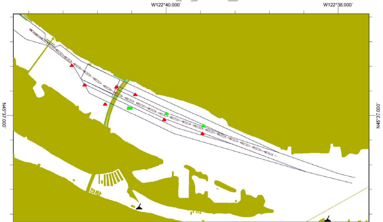
Figure A - 22: Run 22a, 27-ft Channel, Sulphur Guardian Ballast (453ft x 75ft x 19ft) Upbound 10-yr River Flow, Wind S 15 Knots, Pilot B, Proposed CRC Primary Span
