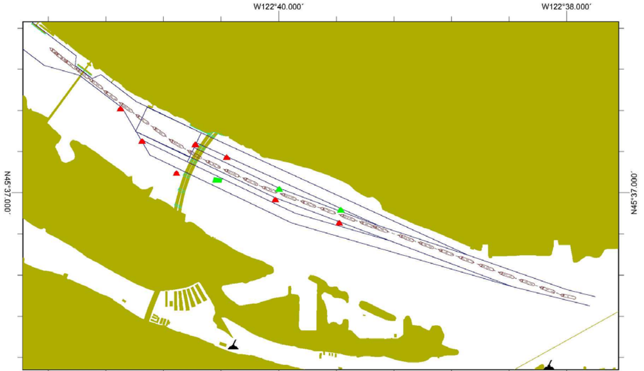
Figure A - 23: Run 22b, 27-ft Channel, Sulphur Guardian Ballast (453ft x 75ft x 19ft) Upbound 10-yr River Flow, Wind S 15 Knots, Pilot A, Proposed CRC Primary Span
