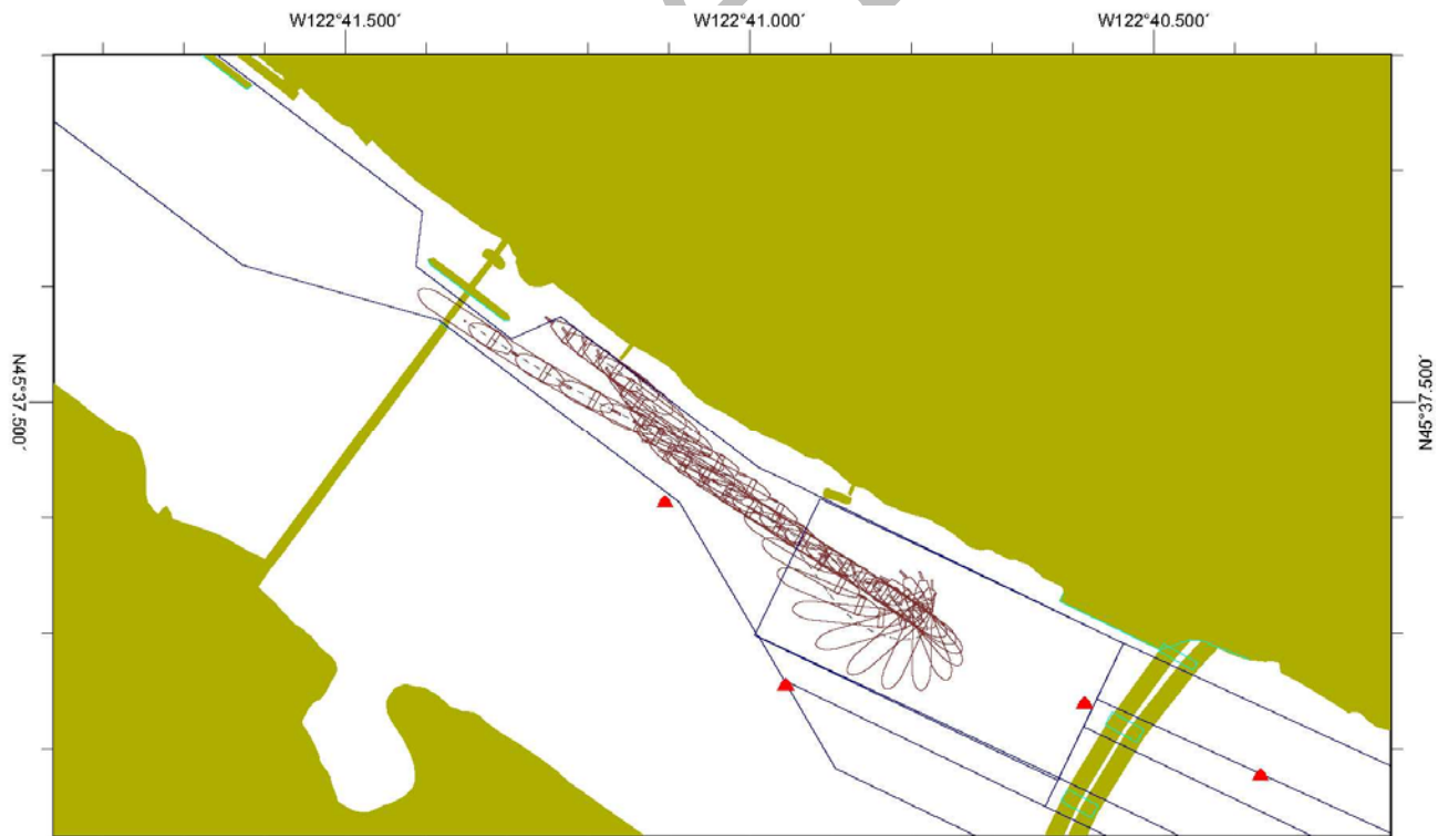
Figure A - 8: Run 9 VTB, Cape Bird Loaded (580ft x 101ft x 33ft) Downbound Turning 10-yr River Flow, Wind S 15 Knots, Two 3000hp Tractor Tugs, Pilot B, Proposed CRC
