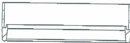
Versa Steel Open End Cutting Shoe and Pipe Cross-Section View
